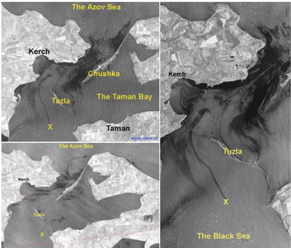
Fig. 6.4.1. Satellite SAR imaging of the Kerch Strait on 16.11.2007, i. e., five days after the catastrophe. Location of the Volgoneft-139 tanker bow part is marked with a cross.
